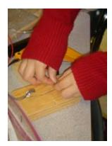
Paper clips should be configured so that one end is wrapped around a push pin while the other end is straightened to create the switch.
