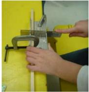
A miter box should be clamped to a table in order for students to saw their wood pieces. Clamps should be used to hold the wooden pieces in place.
