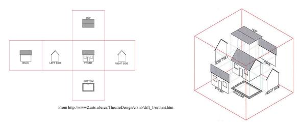
Isometric Drawing is a form of 3-D drawing in which there are three types of lines: vertical lines, 30° lines to the right and 30° lines to the left. Isometric graph paper makes it easy to draw neat, accurate images of design ideas. See the next page for a sample.
